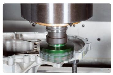
$\bullet$  A 25 HP machine can mount a  $\phi$  125 mm cutter
